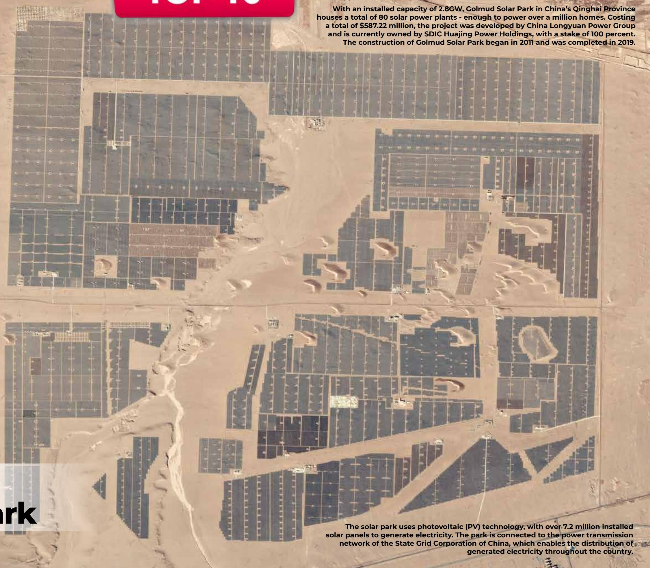
The solar park uses photovoltaic (PV) technology, with over 7.2 million installed solar panels to generate electricity. The park is connected to the power transmission network of the State Grid Corporation of China, which enables the distribution of generated electricity throughout the country.
